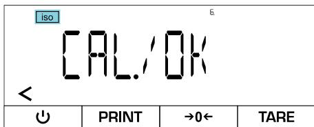
⇒ When the adjustment is complete, <CAL./OK> appears on the display
