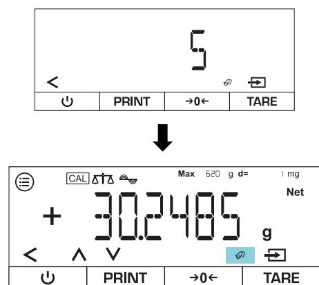
⇒ Measurement is performed and the remaining number of measurement cycles is displayed (in the example = 5 cycles)
