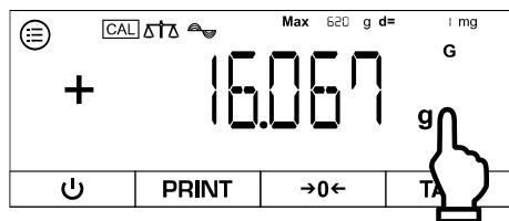
⇒ Touch the weighing unit field (quick access must be activated → see Chap. 10.2.1)
