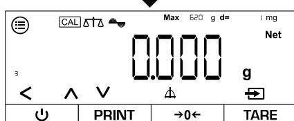
⇒ Weight value is saved (the number at the bottom left shows the number of weighings)
