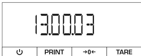
⇒ The scales switch to standby mode and display the set time
