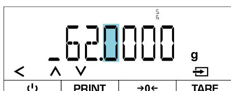
⇒ Enter the weight value of the external calibration weight (for numerical input, see Chap. 3.2.2)
